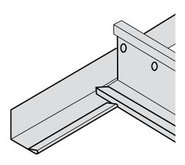
Where the grid is laid on top of the perimeter trim, the gasket of the perimeter trim needs to be cut and removed.
