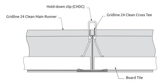
In case of high air pressure from below, hold-down clips need to be used to avoid uplift of tiles and to provide airtightness.
